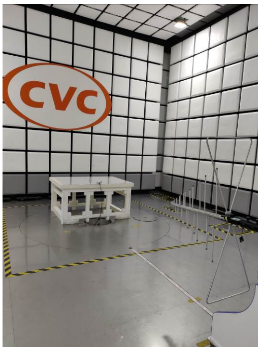
(2) Radiated spurious emission Test Setup-2(Below 1GHz)
