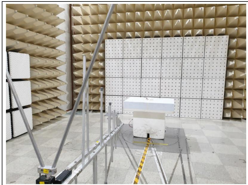
**3. Photo of Radiated Spurious Emission Test (Above 1 GHz)**
