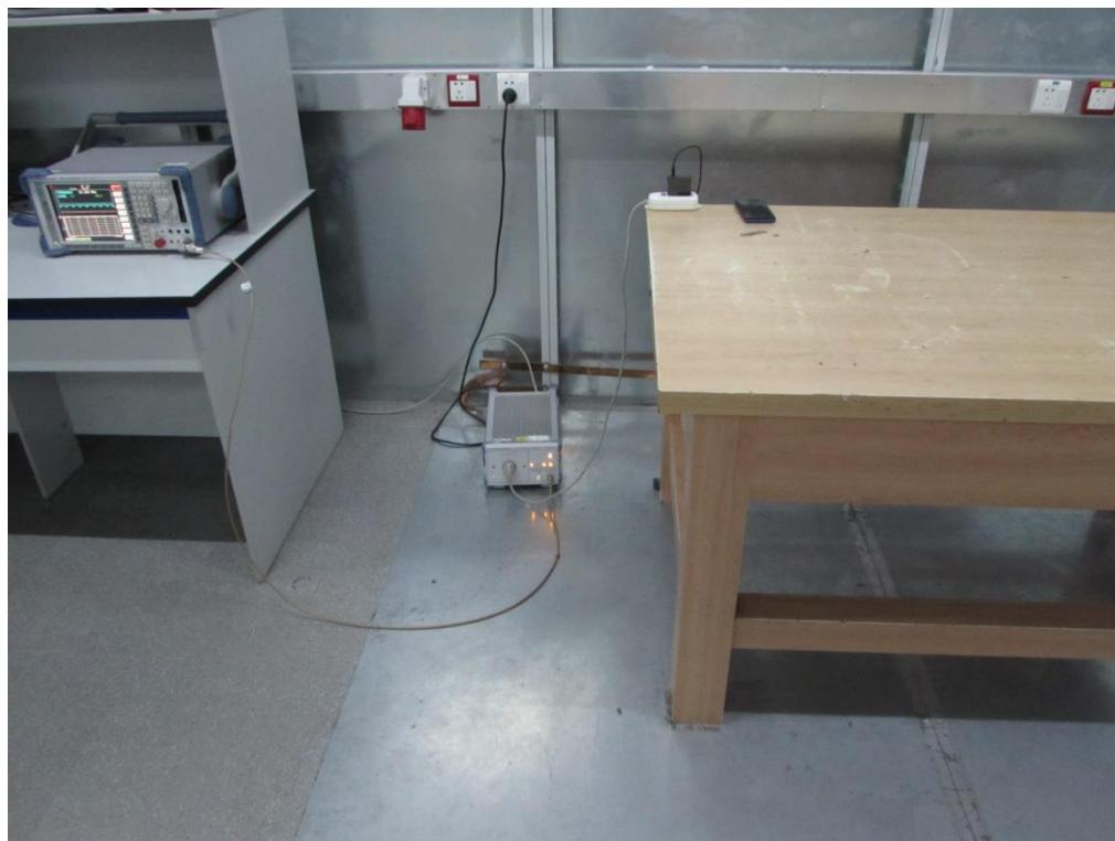
Radiated Emission From 9kHz to 30MHz
