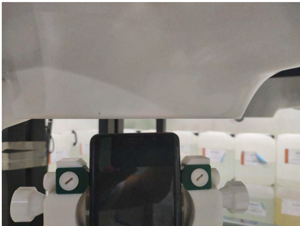
Body top side(separation distance is 10mm)
