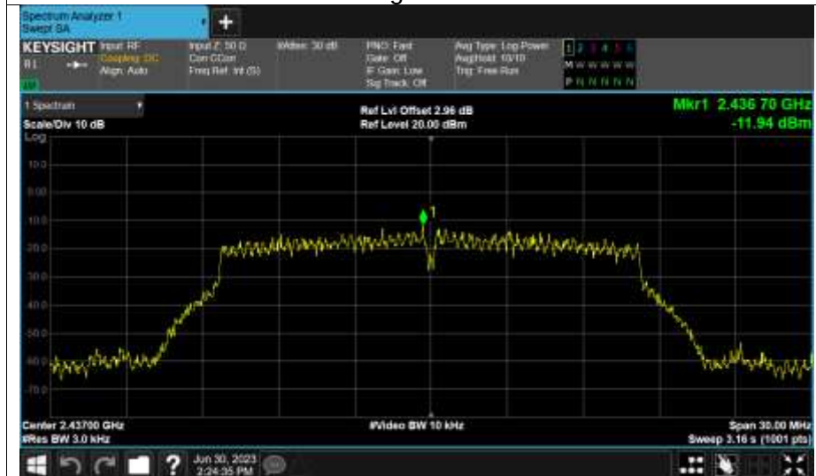
PSD NVNT g 2462MHz Ant2
