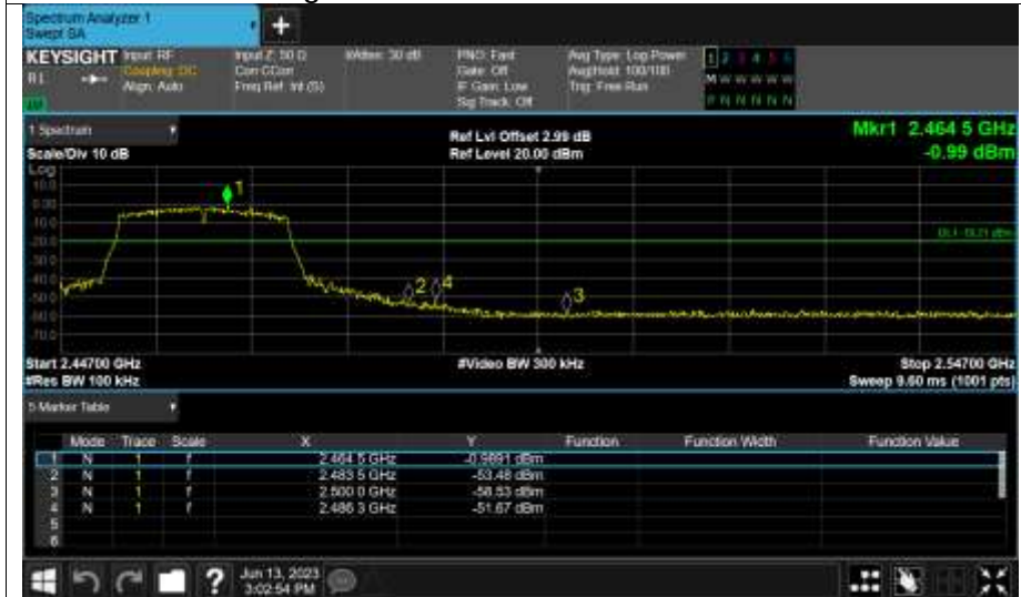
Band Edge NVNT n20 2412MHz Ant2 Ref
