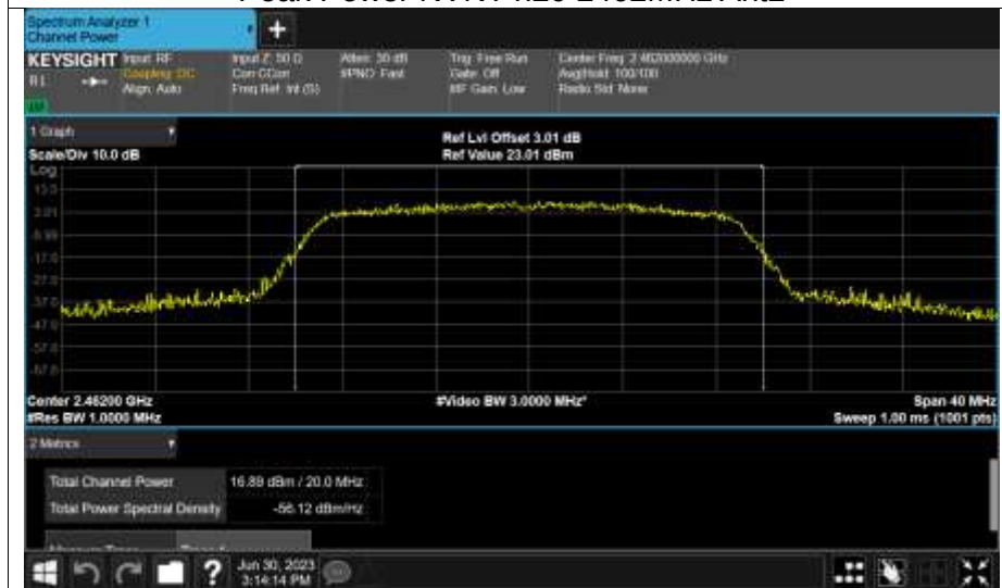
Peak Power NVNT n20 2462MHz Ant2
