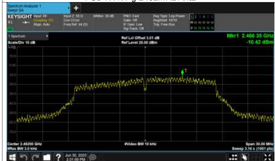
PSD NVNT g 2462MHz Ant2
