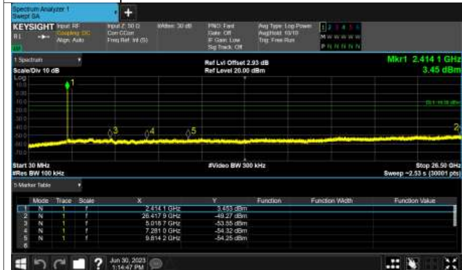
Tx. Spurious NVNT b 2437MHz Ant2 Ref
