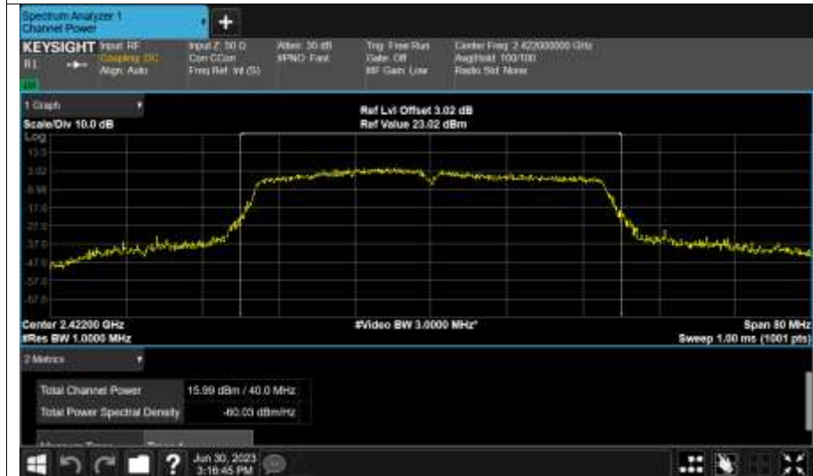
Peak Power NVNT n40 2422MHz Ant2
