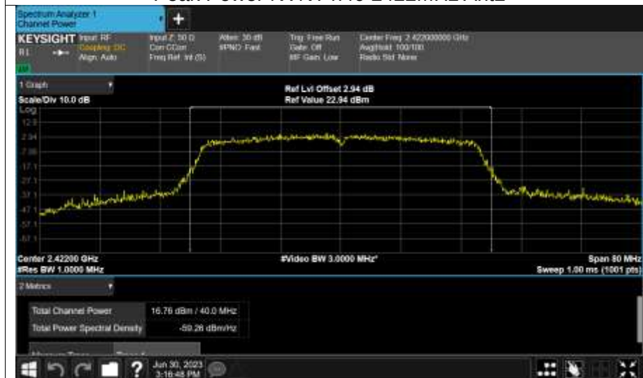
Peak Power NVNT n40 2437MHz Ant1
