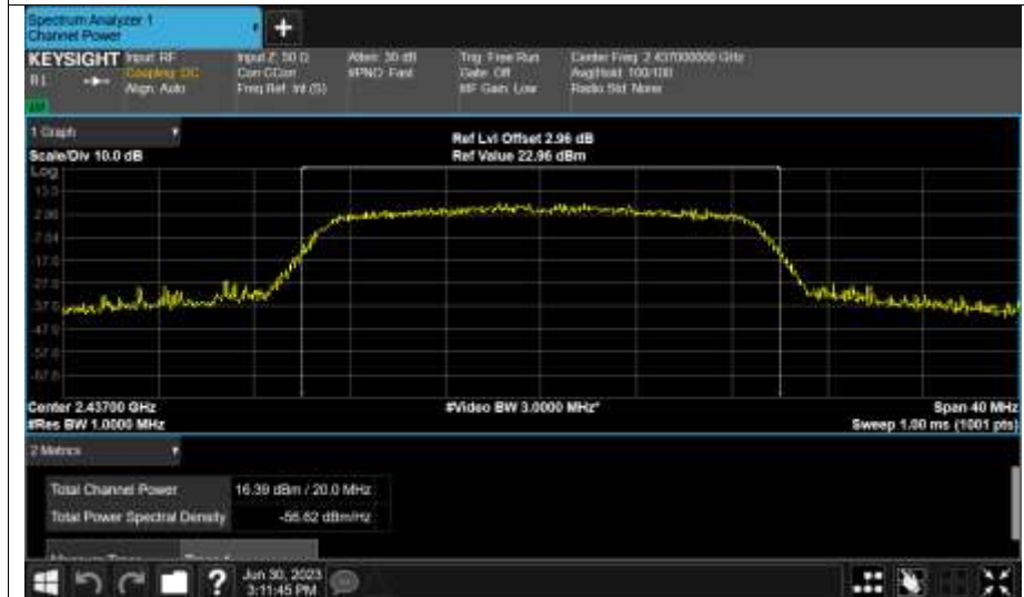
Peak Power NVNT n20 2462MHz Ant1
