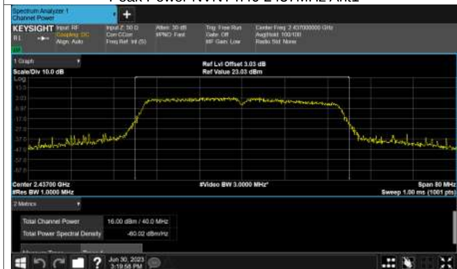
Peak Power NVNT n40 2437MHz Ant1
