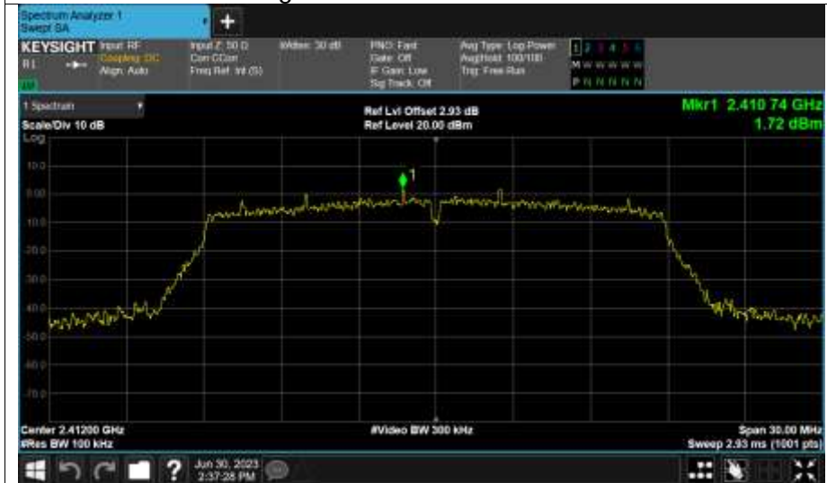
Band Edge NVNT n20 2412MHz Ant2 Ref
