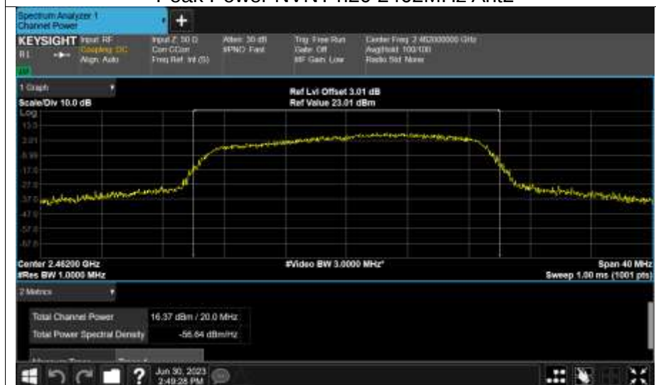
Peak Power NVNT n20 2462MHz Ant2
