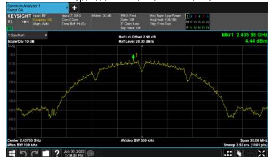
Tx. Spurious NVNT b 2437MHz Ant2 Ref
