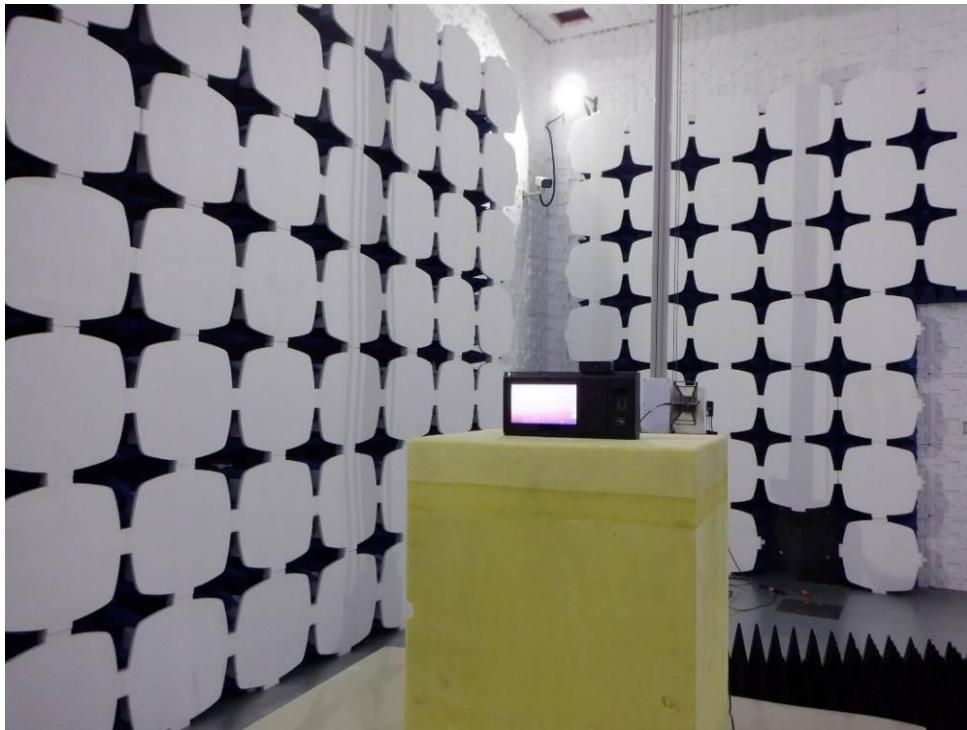
**Conducted Emissions at AC Power Line (150kHz-30MHz)**
