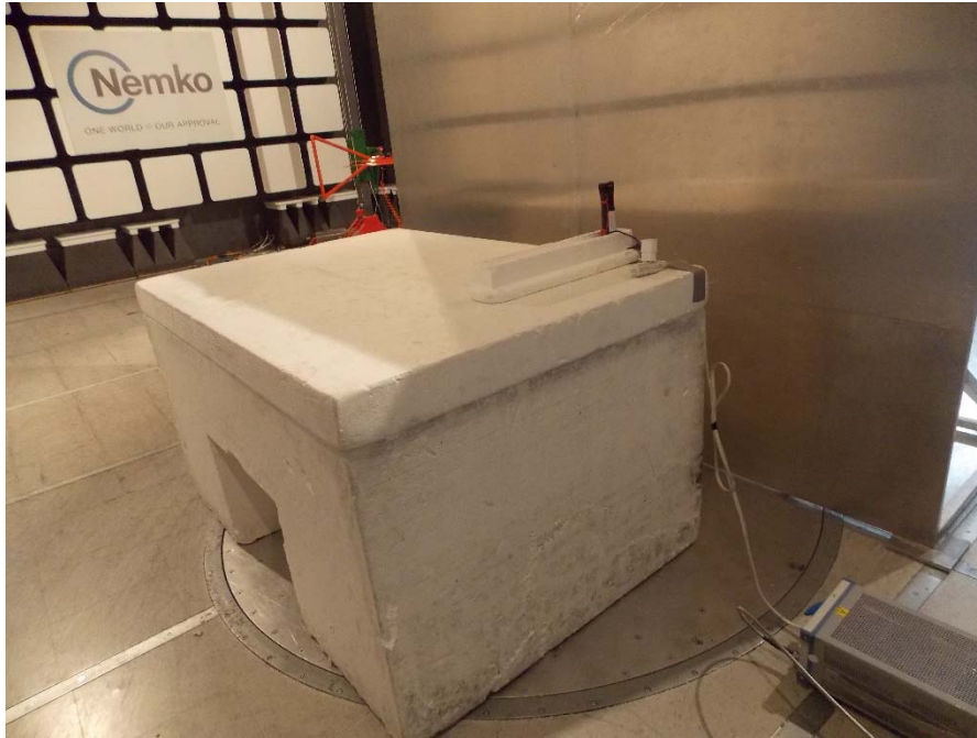
Conducted emissions – from AC mains power ports setup photo
