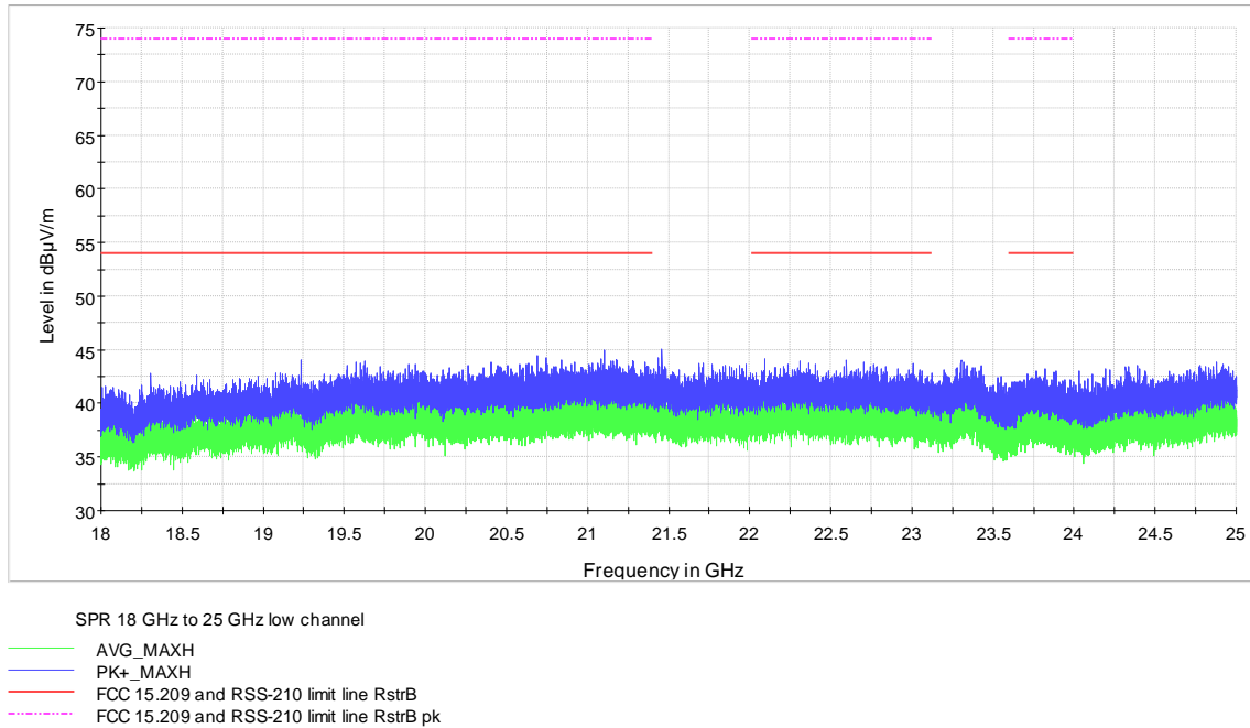
Figure 7.6-48: radiated spurious emissions from 18 GHz to 25 GHz on 802.11g (54 Mbps) at low channel
