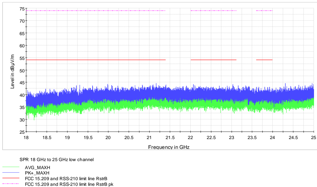
Figure 7.6-9: radiated spurious emissions from 18 GHz to 25 GHz on 802.11b (1 Mbps) at low channel
