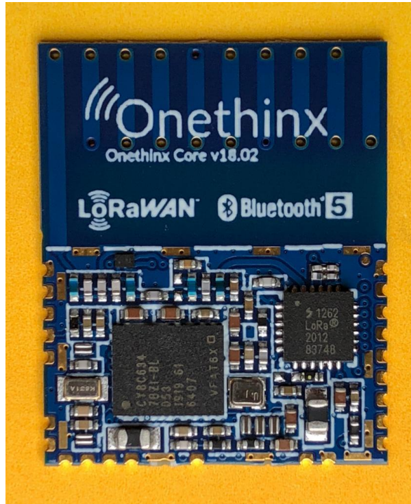
LoRaWAN Module without Shielding Top View
