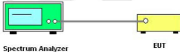
The EUT which is powered by the Battery, is connected to the Spectrum Analyzer; the RF load attached to the EUT antenna terminal is 50 Ohm; the path loss as the factor is calibrated to correct the reading. Make the measurement with the spectrum analyzer's resolution bandwidth(RBW) = 100 kHz. In order to make an accurate measurement, set the span greater than RBW.
