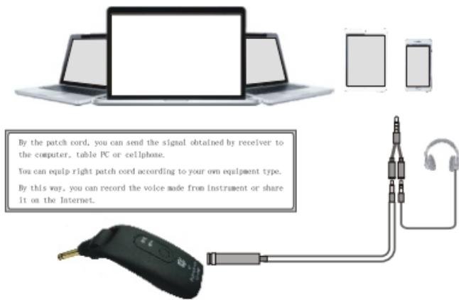
By the patch cord, you can send the signal obtained by receiver to the computer, table PC or cellphone.
