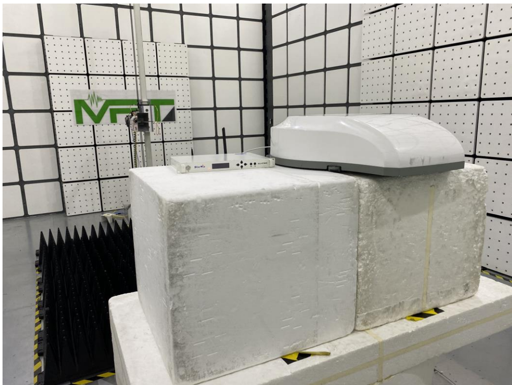
Description: Radiated Spurious Emission Test Setup for 1GHz ~ 18GHz
