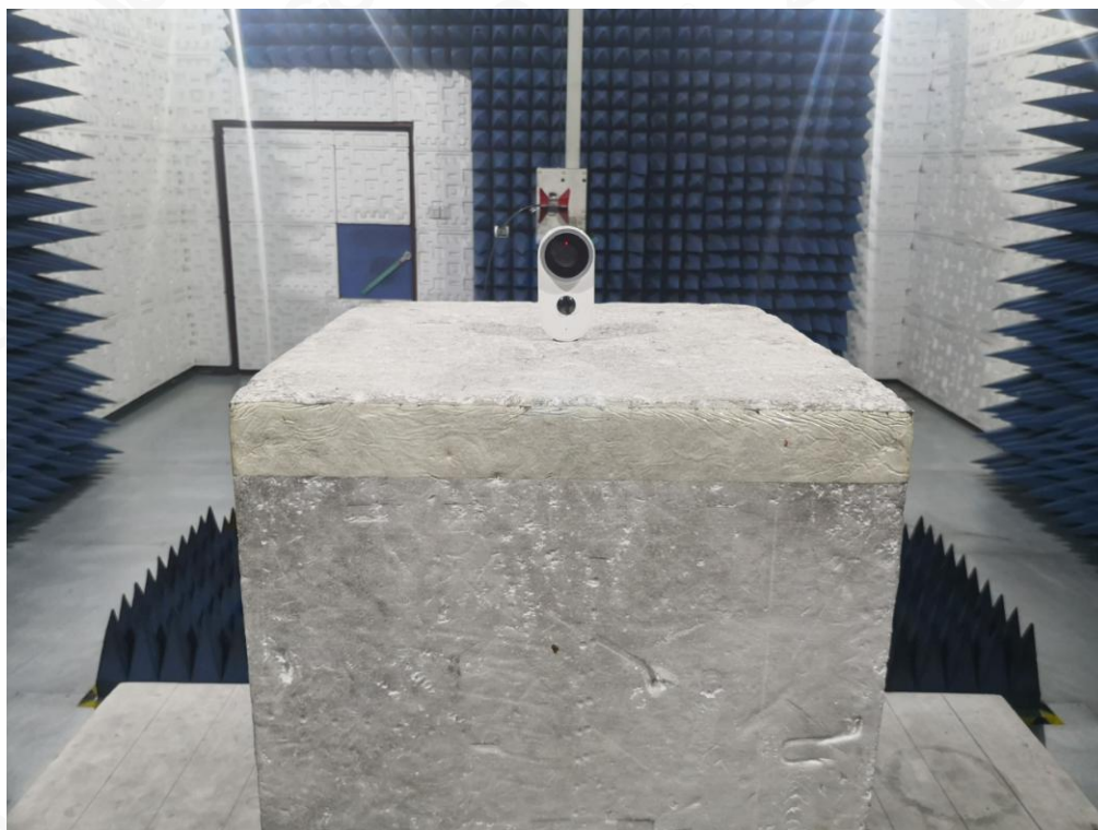
FCC RADIATED EMISSION TEST SETUP ABOVE 1GHZ
