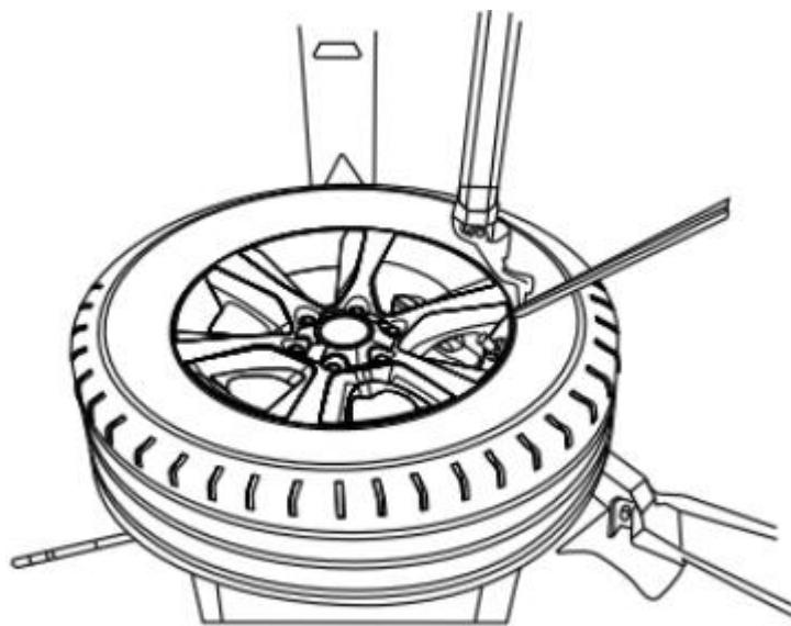
Clamp the tire onto the tire changer, adjust the valve to the 1 o'clock position relative to the tire separation head, insert the tire tool and lift the tire bead onto the mounting head to remove the bead.
