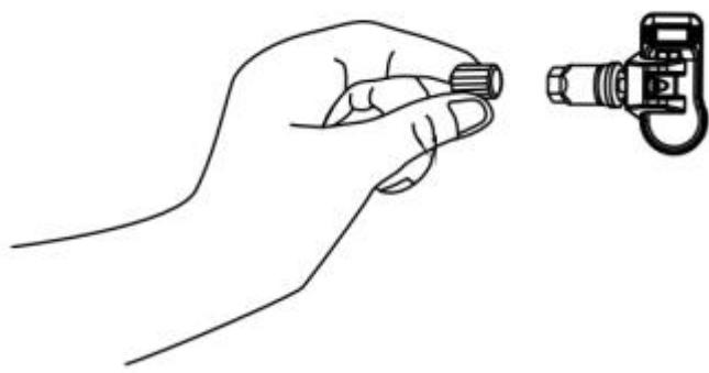
Step 1. Remove the valve caps and nuts from the valve stems one by one.
