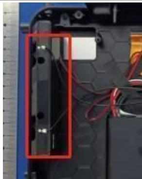
The antenna is FPC antenna.5.1G:3.73dBi,5.8G:4.55dBi
