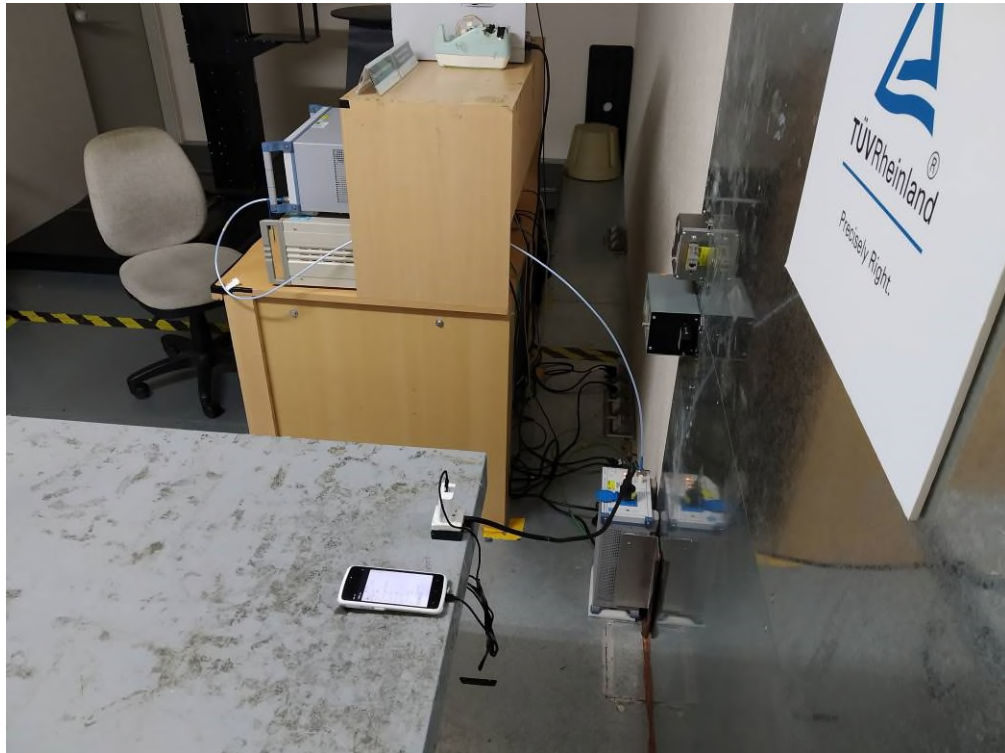
Photograph 5: Set-up for for AC Mains (Front)
