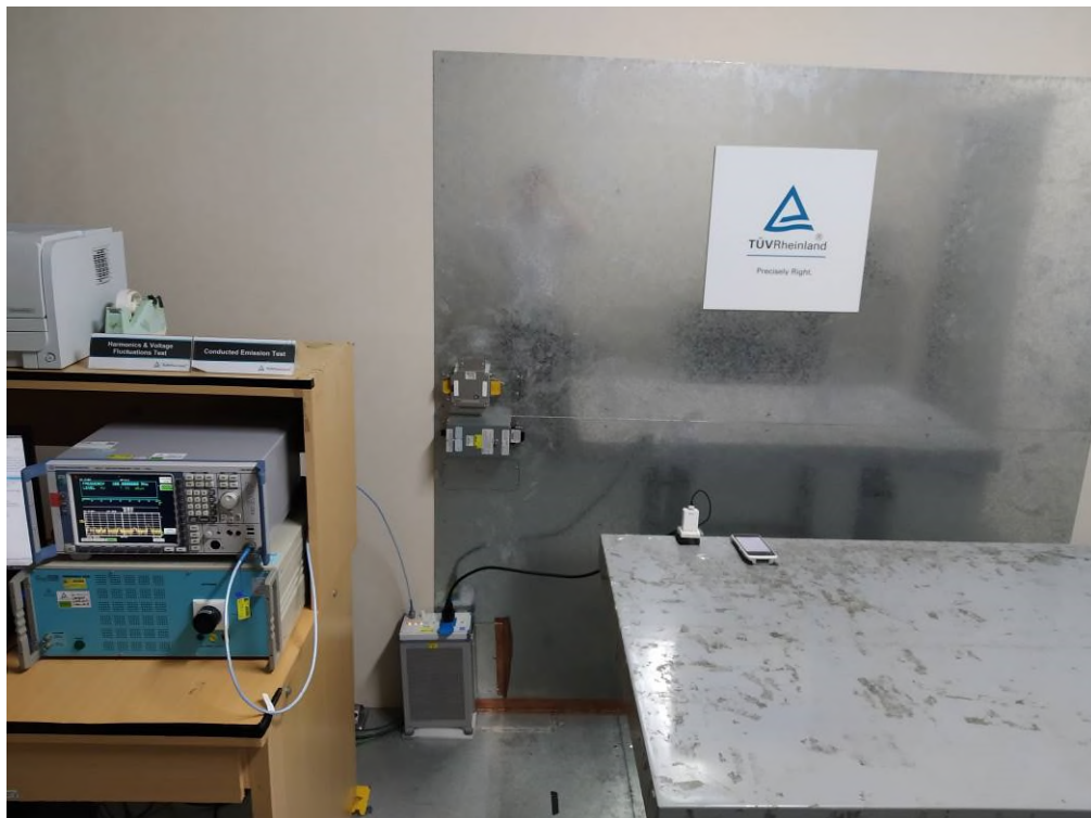
Photograph 5: Set-up for for AC Mains (Front)
