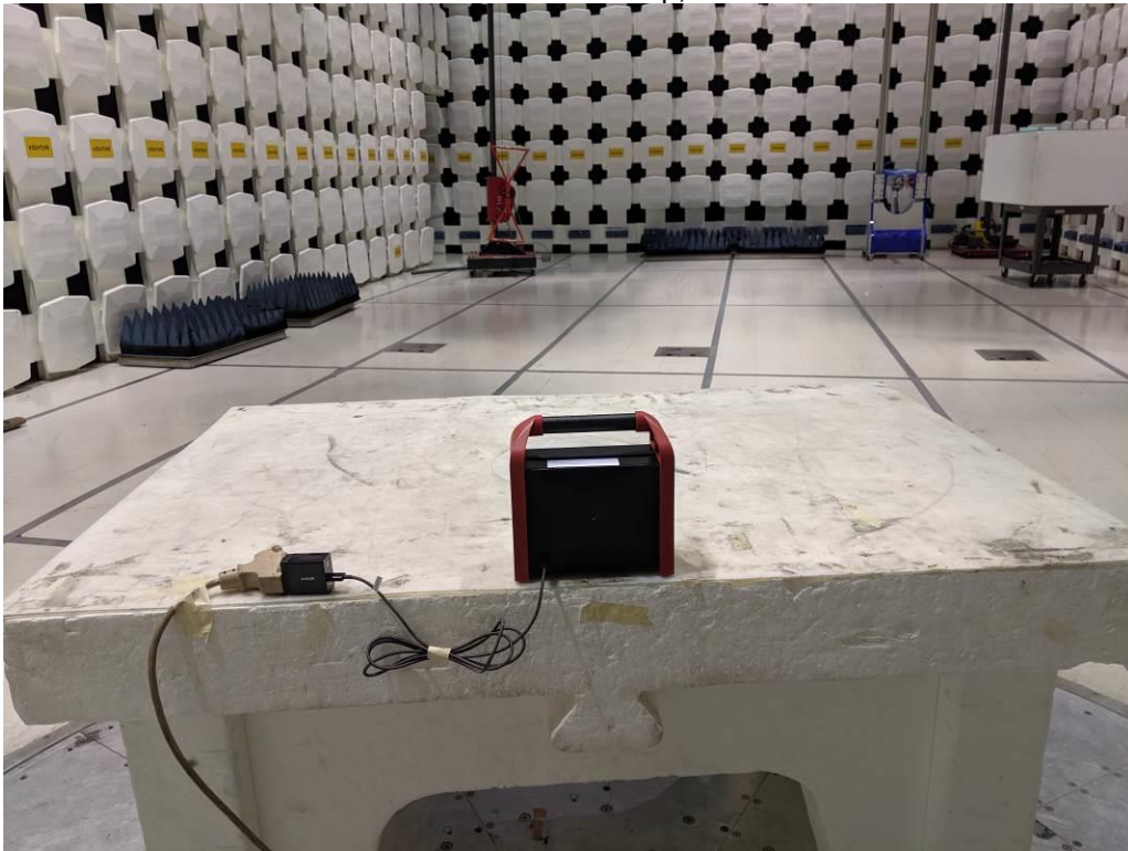
Radiated Emissions Test Setup, 30-1000 MHz
