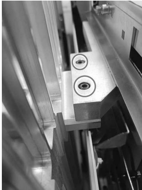
Upper connector - screws to be tightened
