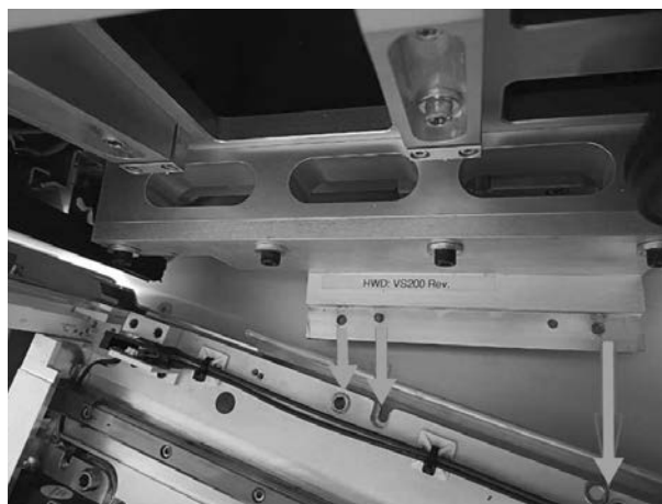
Lower connector - attachment points
