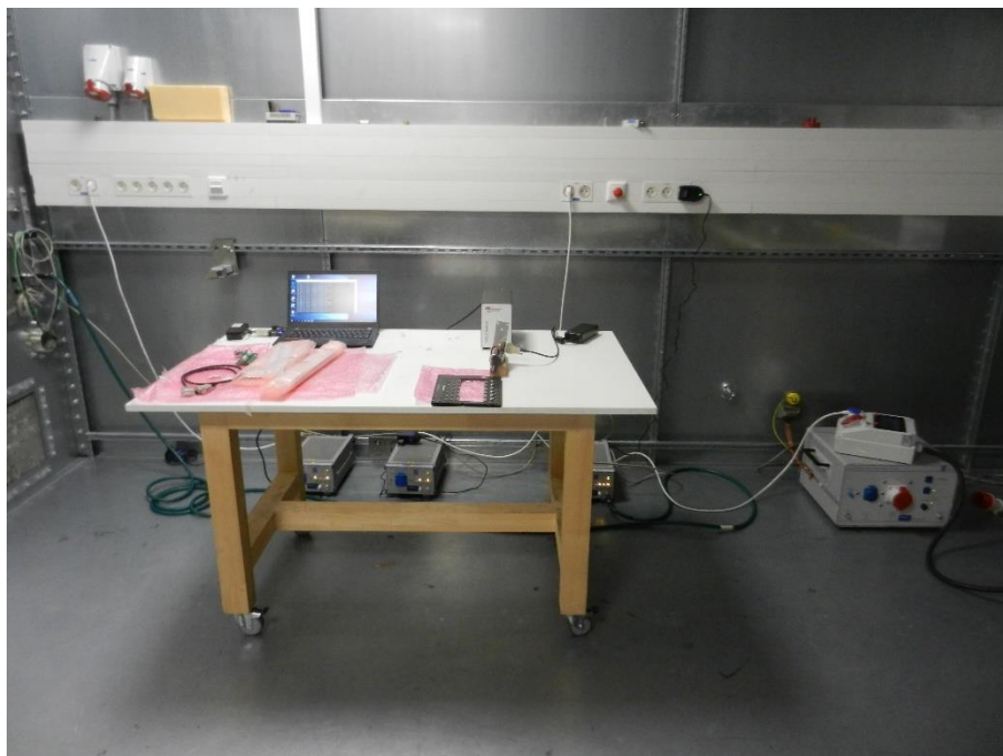
-Conducted AC emissions – Test for Scanner module
