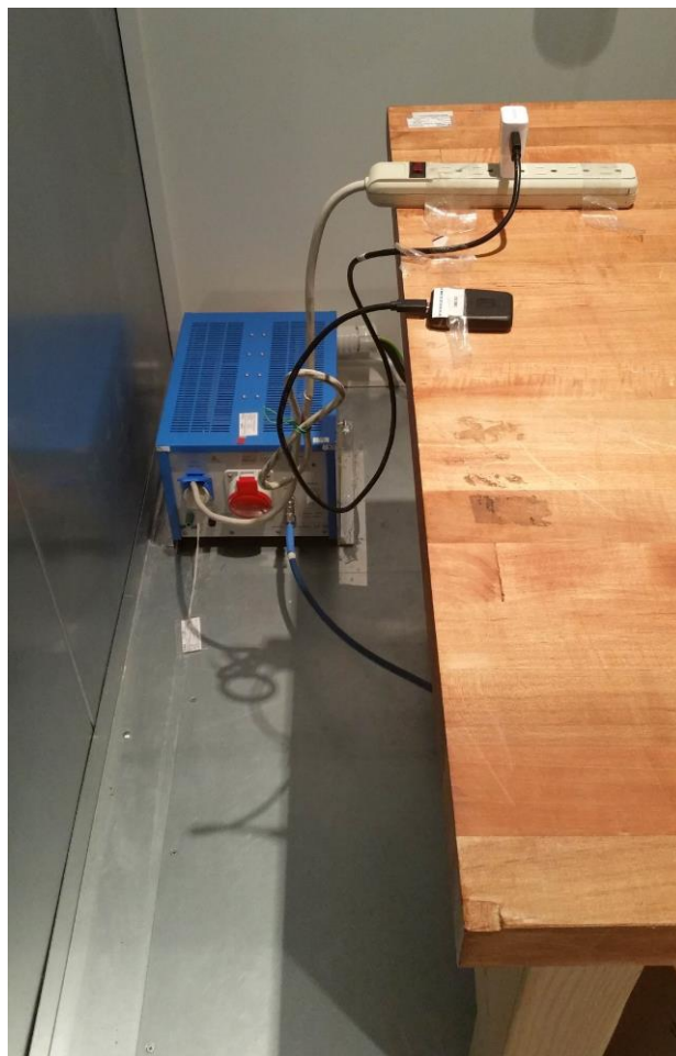
Figure B5: Conducted Emission Test setup
