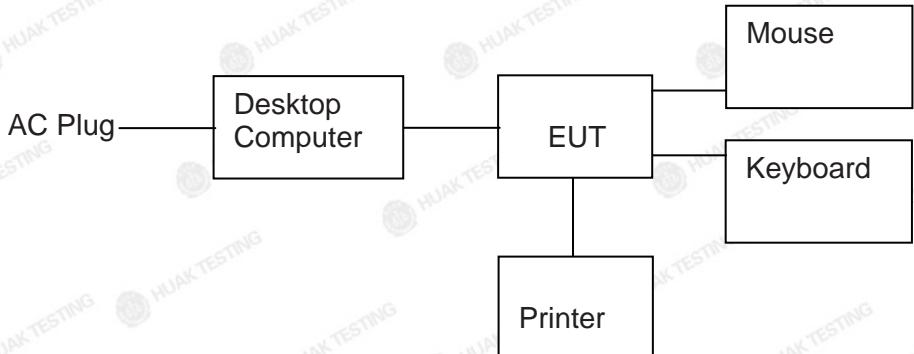
Operation of EUT during Above 1GHz Radiation testing:
