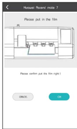
(7) After cutting, the protective film will be pushed out automatically. Take out the protective film and finish cutting.
