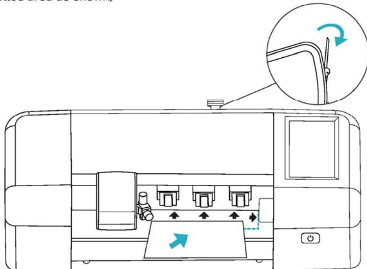
(3) Slowly lift the pressing bar so that the platen roller presses the protective film.
