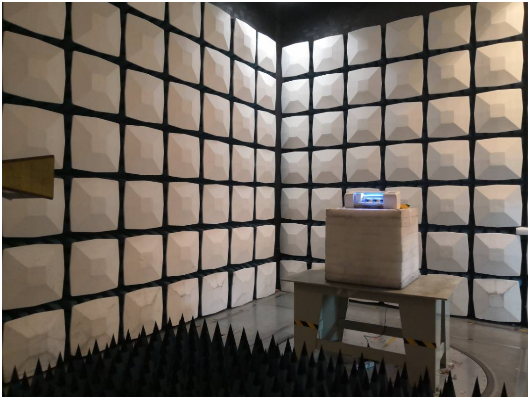
Radiated Emission Above 1GHz View
