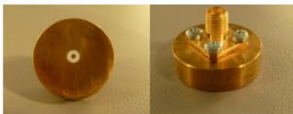
Figure 1 – MVG LIMESAR Dielectric Probe
