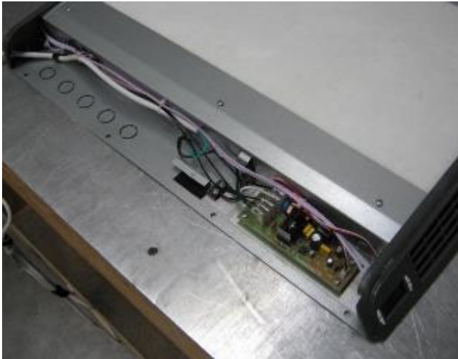
Cover removed, control panel & RF board lower right.
