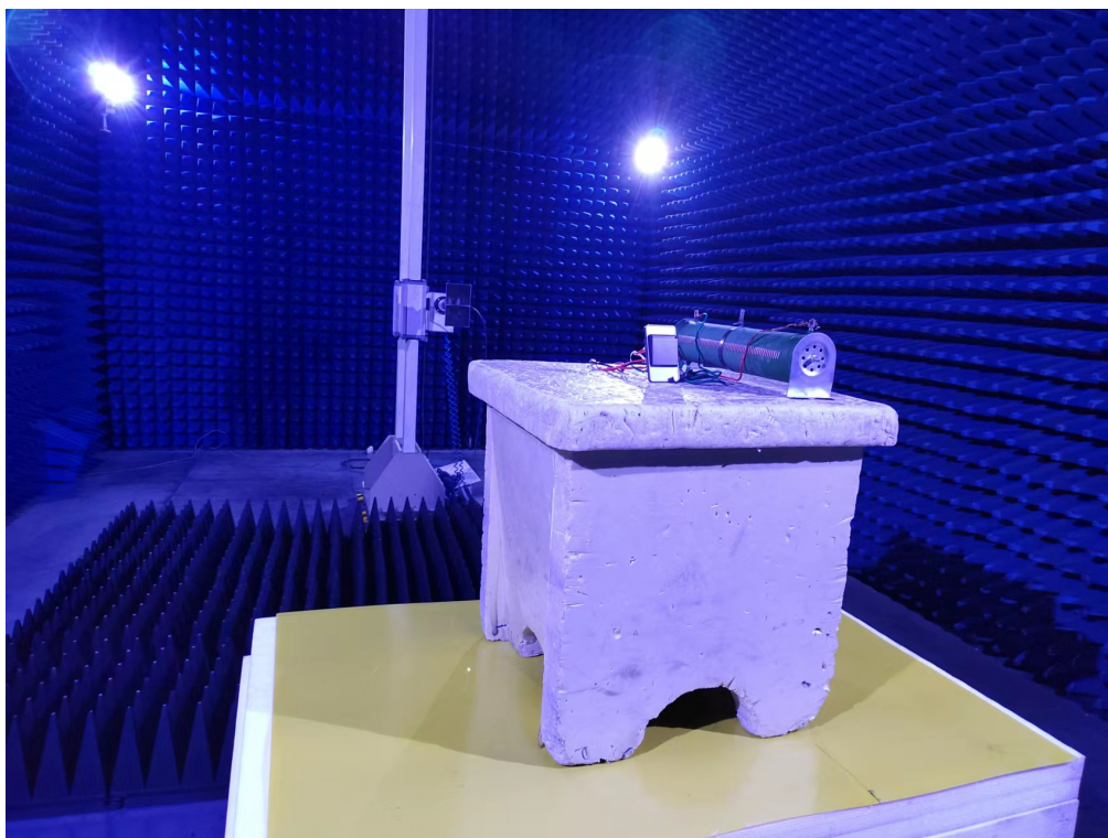
Photo of Radiated Emission Measurement (Above 1 GHz)
