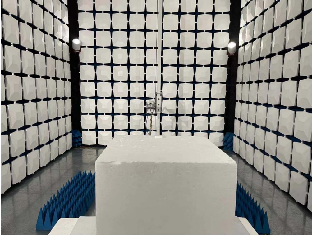
Above 1GHz for radiated emission test setup
