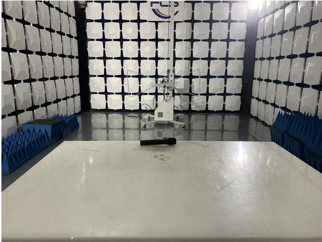
Blow 1GHz for radiated emission test setup
