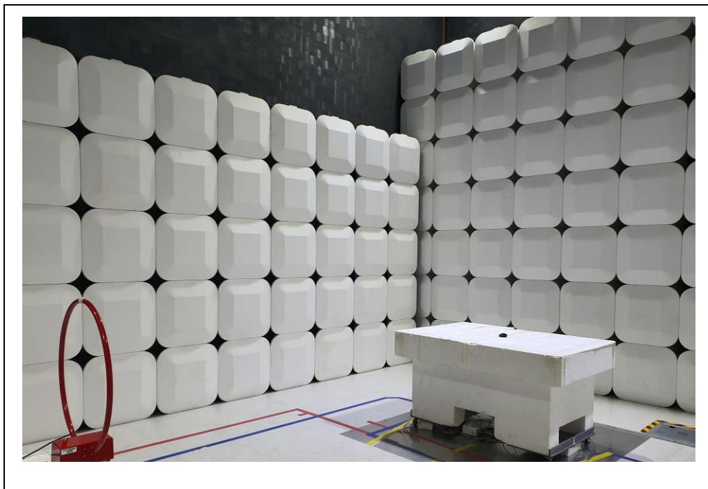
**Test Setup Photo of Radiated Measurement (below 1000MHz))**
