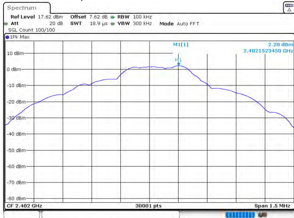
Tx. Spurious NVNT 1-DH5 2402MHz Ant1 Ref
