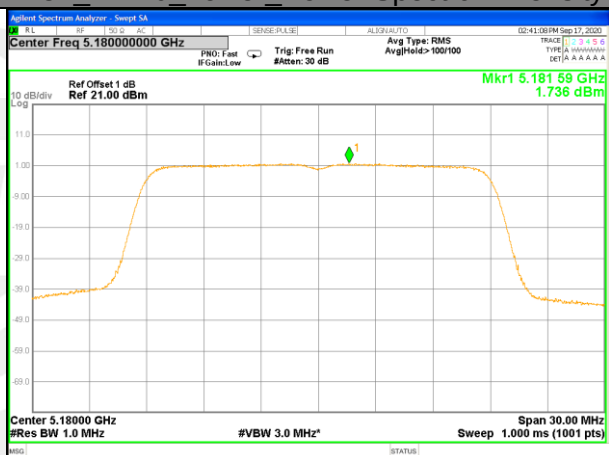
W52_11n20_Higher_Power Spectrum Density
