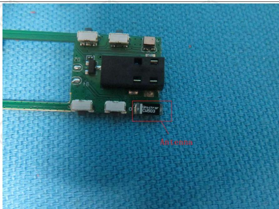
The antenna is integrated on the main PCB and no consideration of replacement. The best case gain of the antenna is 2.64 dBi.
