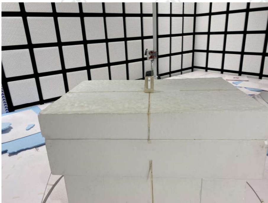
Radiated spurious emission Test Setup-3(Above 1GHz)
