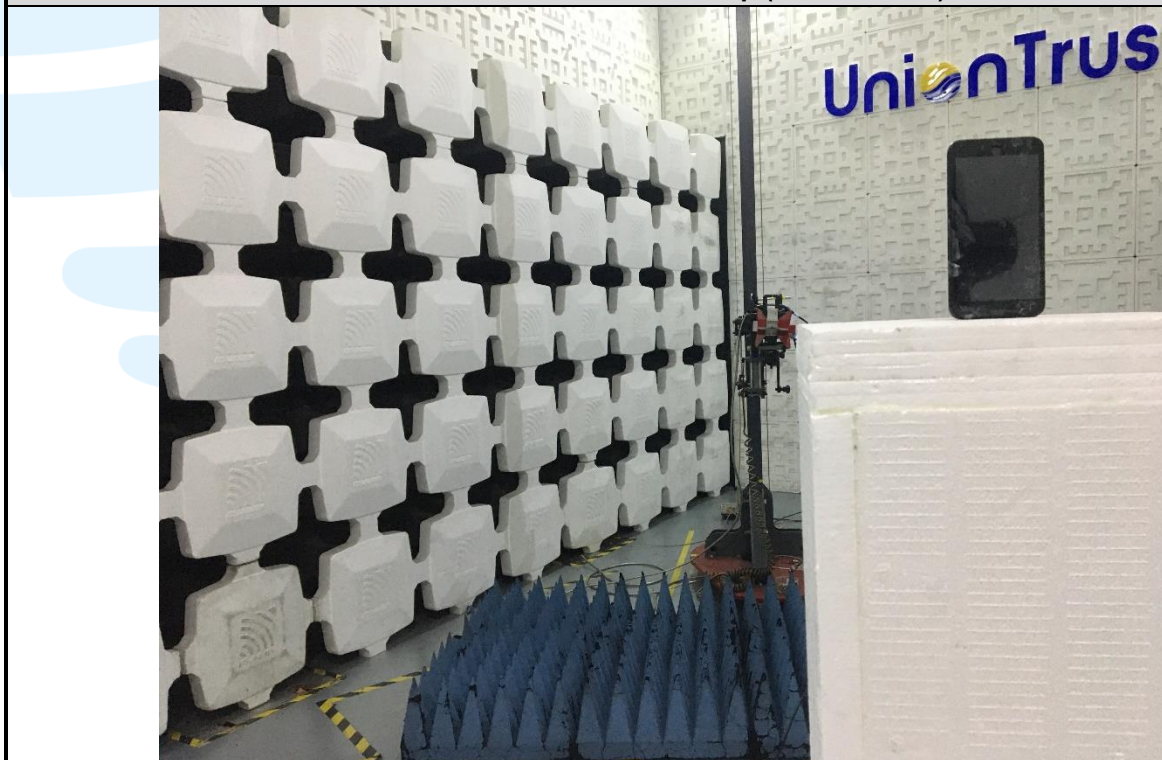
Radiated emission Test Setup (Above 1 GHz)
