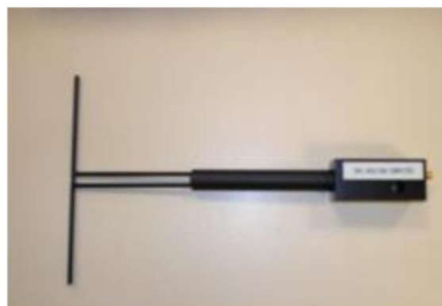
Figure 1 – Satimo COMOSAR Validation Dipole
