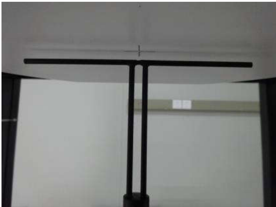
Photo of Dipole Setup
