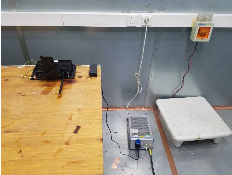
Picture 2: Conducted Emissions Test Setup
