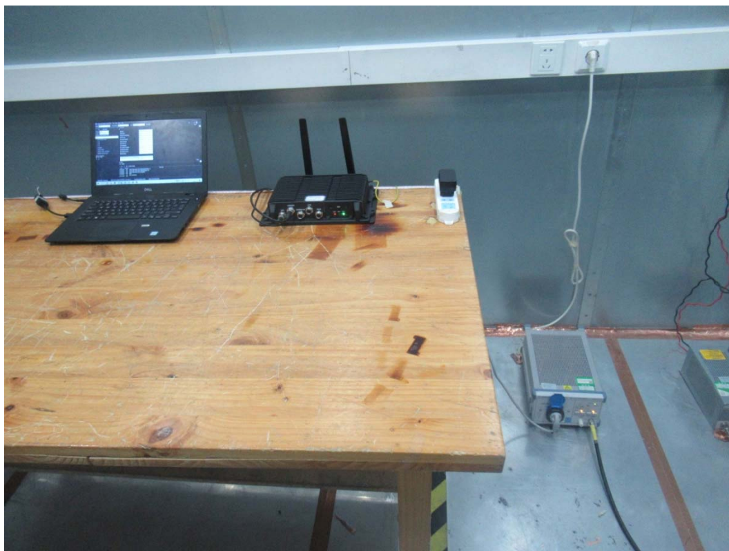
Picture 2: Conducted Emissions Test Setup
