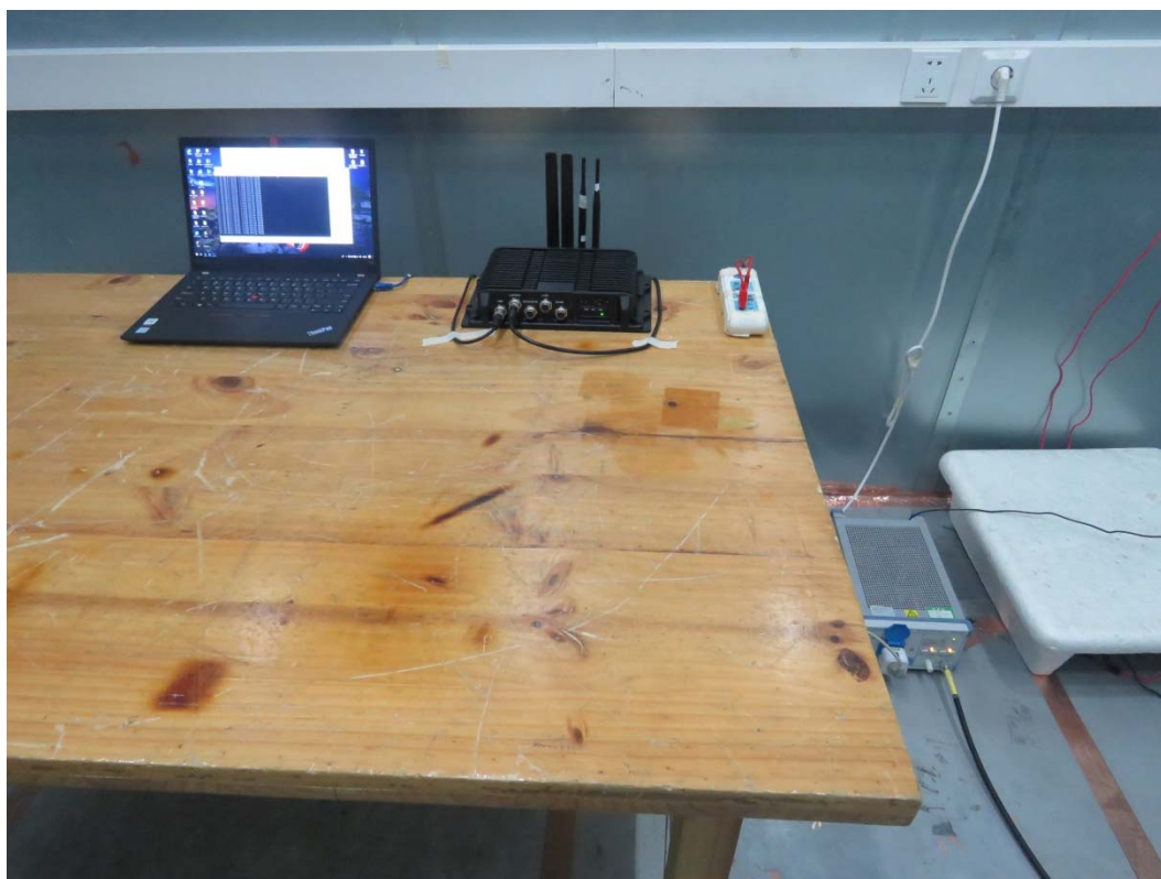
Picture 2 Conducted Emission Test Setup
