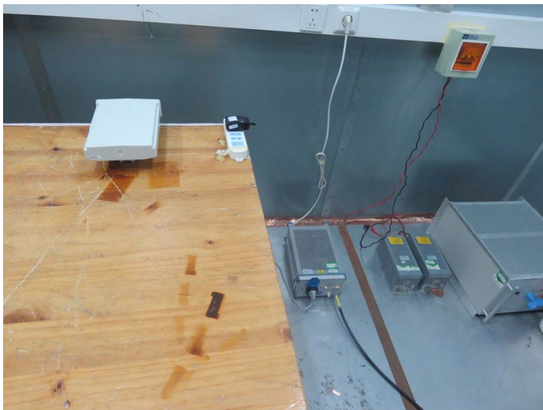
Picture 2: Conducted Emissions Test Setup
