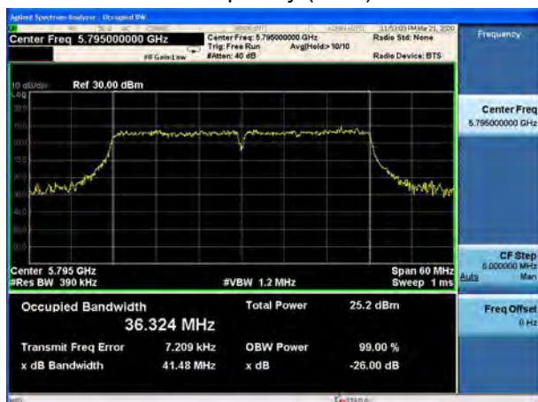
U-NII-3, 802.11ac VHT40 Carrier frequency (MHz): 5755
