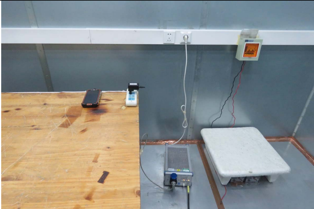
Picture 2 Conducted Emission Test Setup
