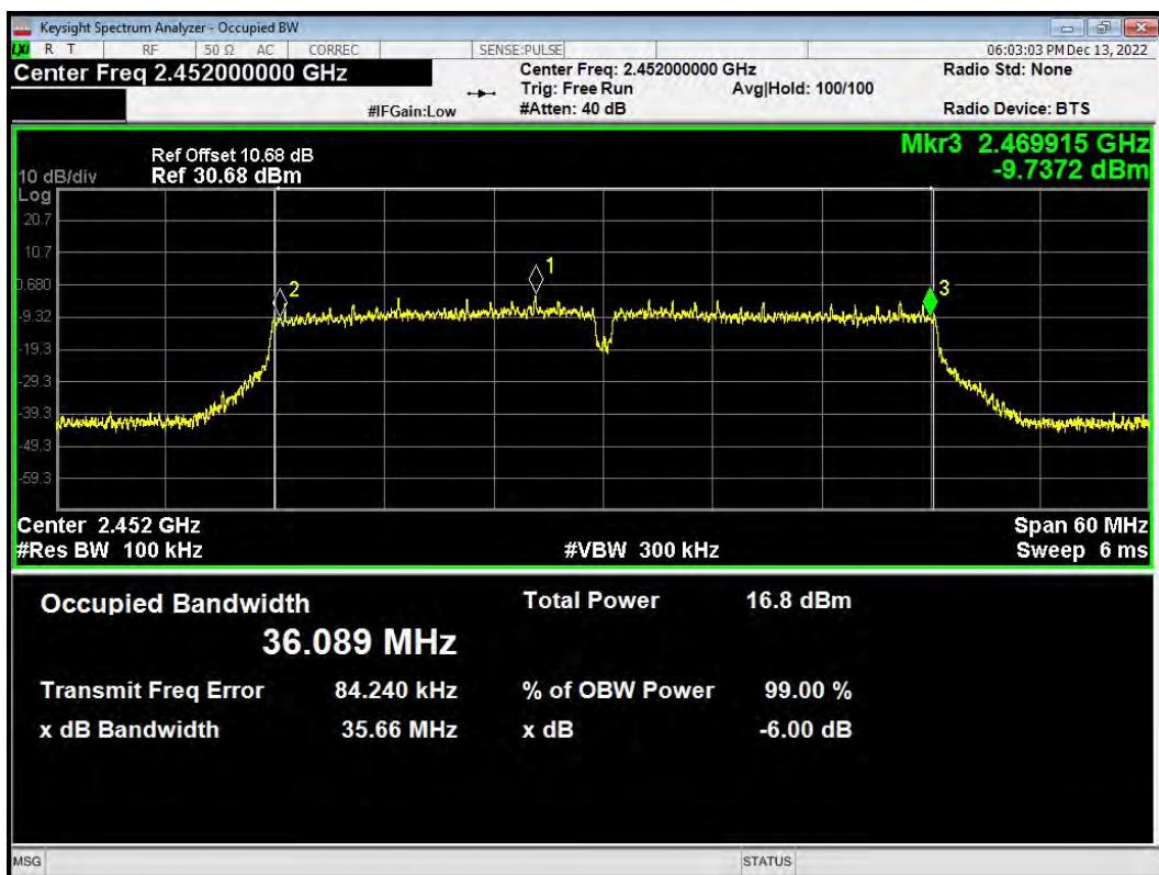
**-6dB Bandwidth BLE(1M) 2402MHz**
