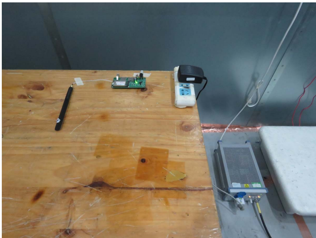
Picture 2 Conducted Emission Test Setup
