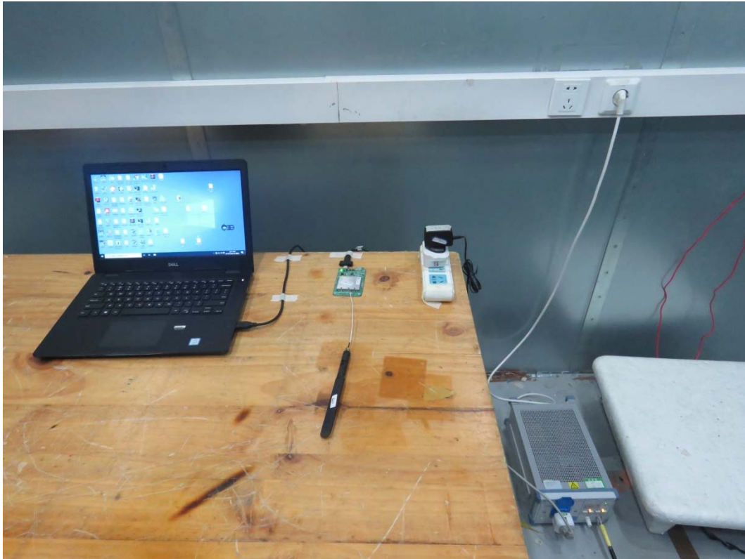
Picture 2 Conducted Emission Test Setup
