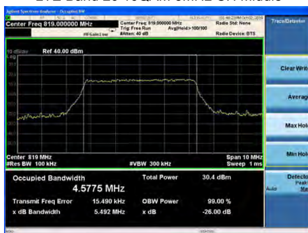
LTE Band 26 16QAM 5MHz CH Middle
