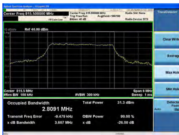
LTE Band 26 16QAM 3MHz CH Middle
