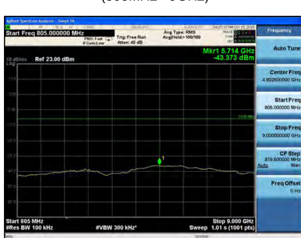
LTE Band 14 16QAM 5MHz 1 RB CH- High (805MHz~ 9GHz)
