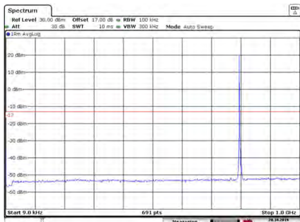
LTE Band 14 5MHz CH-High 9kHz~1GHz
