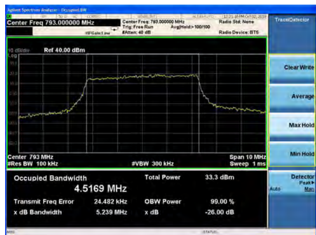
LTE Band 14 QPSK 10MHz CH-Middle
