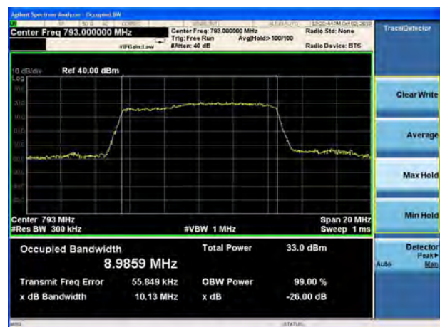
LTE Band 14 QPSK 10MHz CH-Middle
