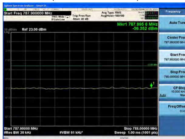
LTE Band 14 QPSK 10MHz 100%RB CH- High (799MHz ~805MHz)
