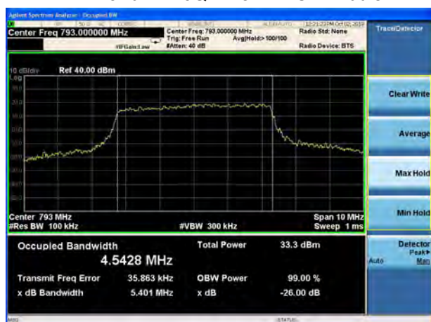
LTE Band 14 16QAM 10MHz CH-Middle
