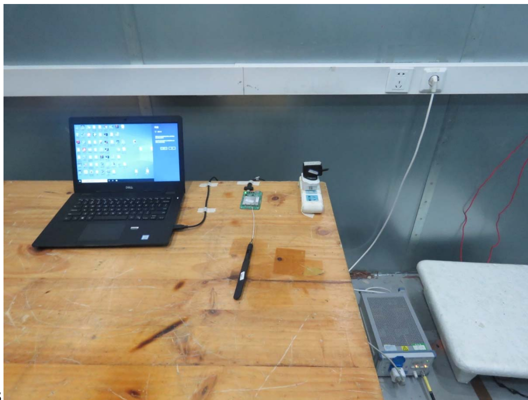
Picture 2 Conducted Emission Test Setup
