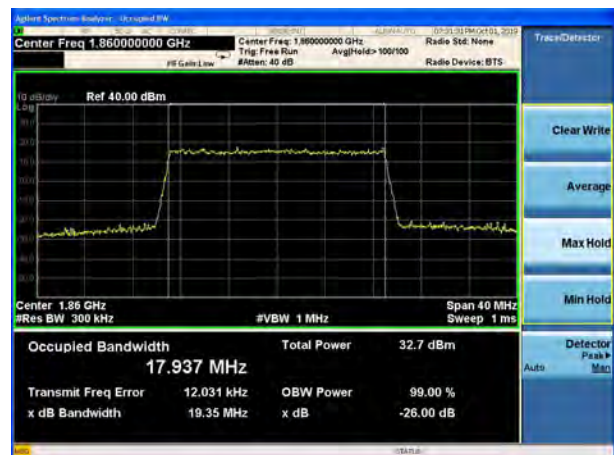
LTE Band 2 20MHz QPSK CH-Middle
