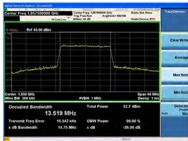
LTE Band 2 15MHz 16QAM CH-Middle
