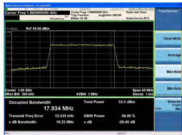
LTE Band 25 20MHz QPSK CH-Middle
