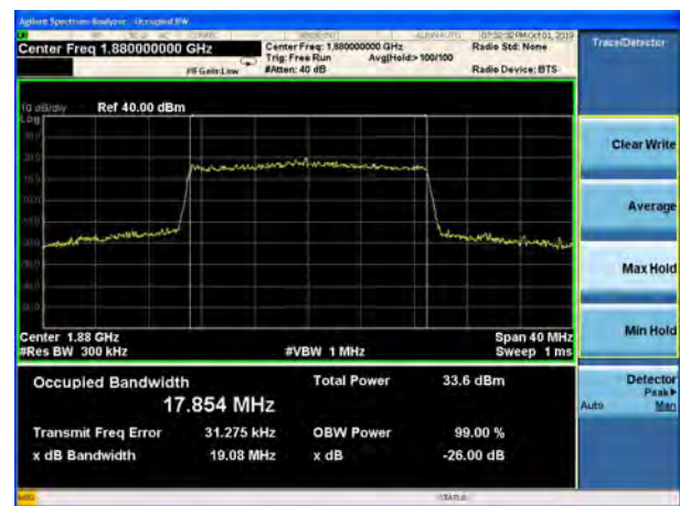
LTE Band 2 20MHz 16QAM CH-High
