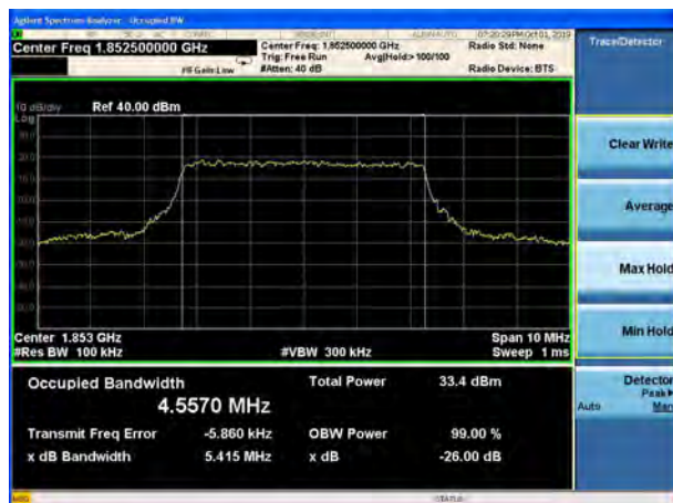
LTE Band 2 5MHz 16QAM CH-Middle
