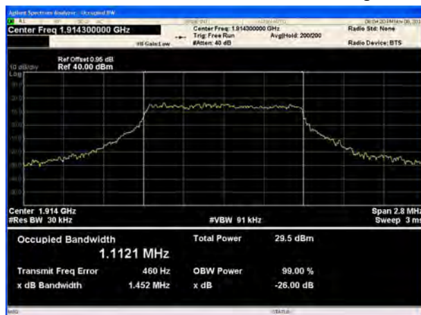
LTE Band 25 1.4MHz 64QAM CH-High
