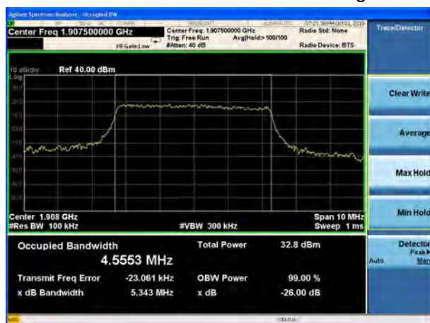
LTE Band 2 5MHz 16QAM CH-High
