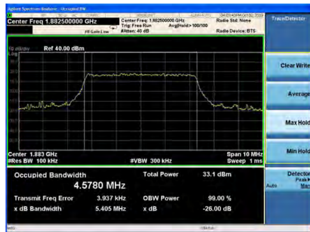
LTE Band 25 5MHz 16QAM CH-High
