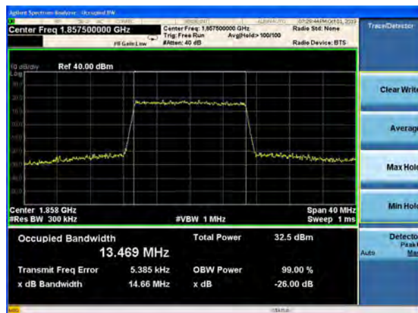
LTE Band 2 15MHz QPSK CH-Middle
