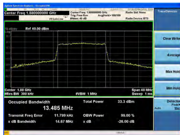
LTE Band 2 15MHz 16QAM CH-High
