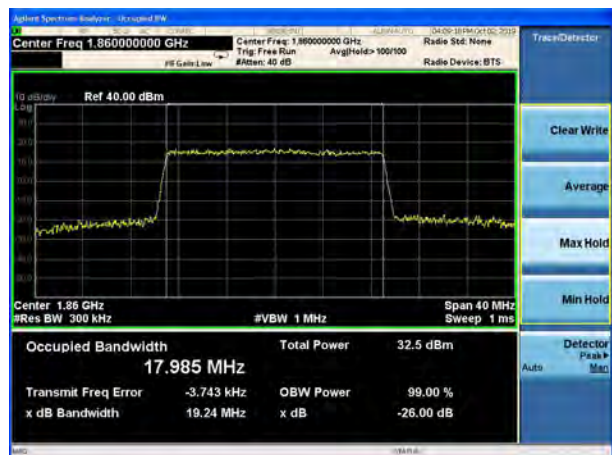
LTE Band 25 20MHz 16QAM CH-Middle
