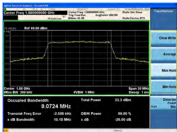
LTE Band 2 10MHz 16QAM CH-High
