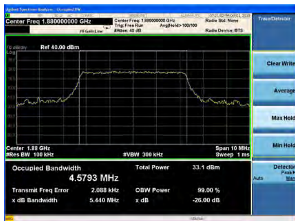
LTE Band 2 5MHz 16QAM CH-High
