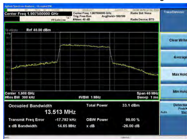
LTE Band 25 15MHz 16QAM CH-High
