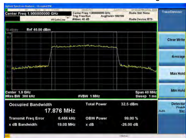
LTE Band 2 20MHz 16QAM CH-High
