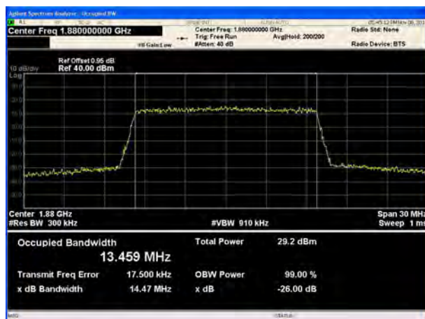
LTE Band 2 15MHz 64QAM CH-High
