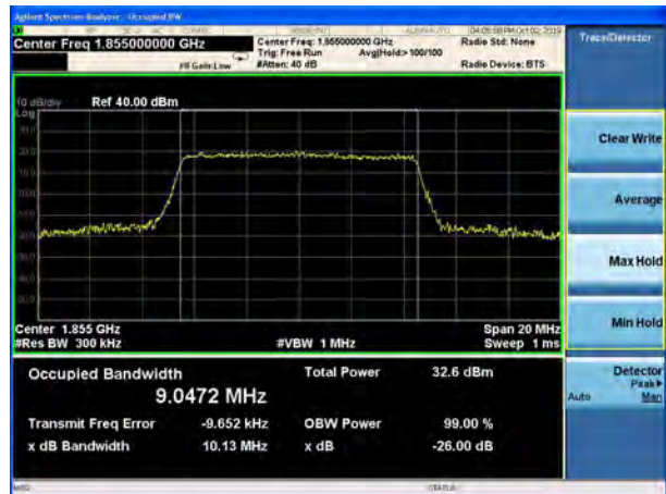
LTE Band 25 10MHz 16QAM CH-Middle
