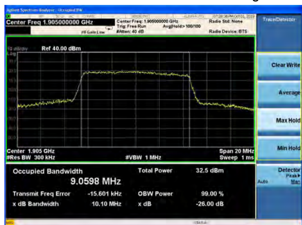
LTE Band 2 10MHz 16QAM CH-High
