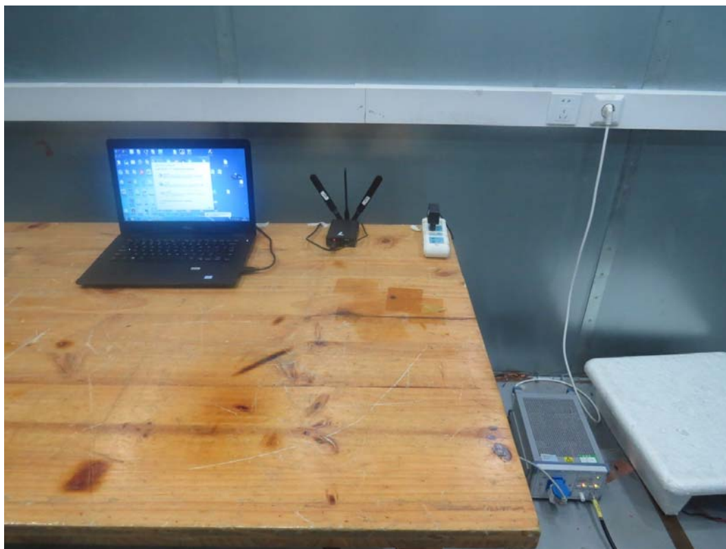
Picture 2 Conducted Emission Test Setup
